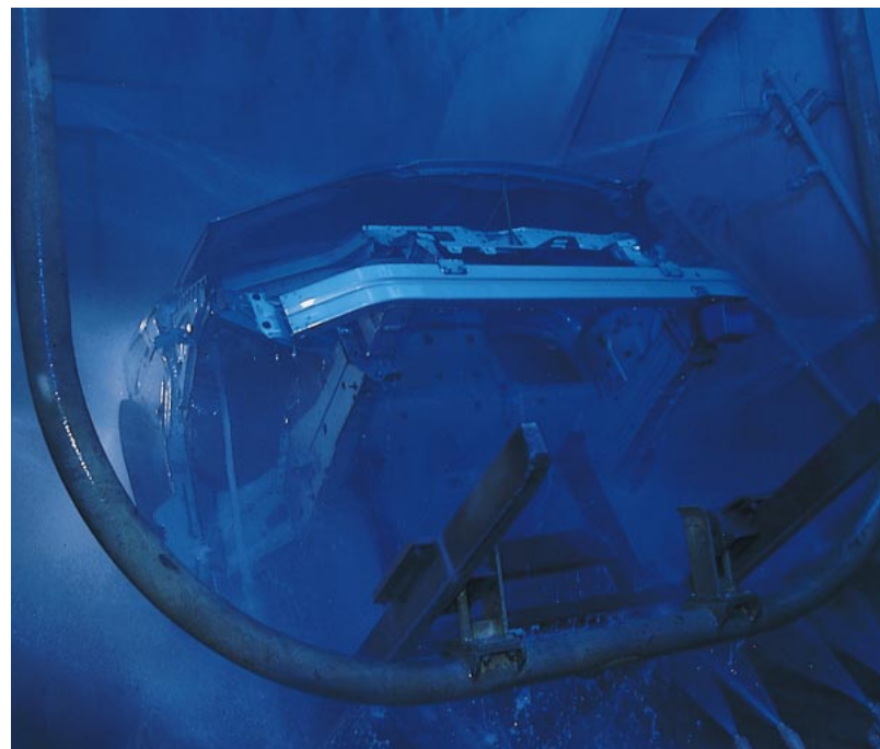
Nickel-free phosphating. This alternative corrosion protection process was developed by Daimler-Chrysler and Henkel Surface Technologies for the production of Mercedes A class cars.
